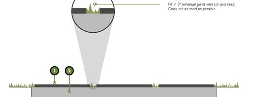
→ Insure sub grade is graded to a 1" in 10' slope and that it is pitched away from any building.
